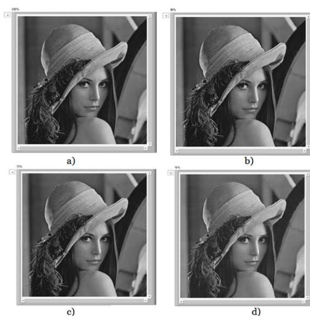
Fig. 7. a) The source image. Reconstructed images when a b) 90% (37.32 dB), c) 75% (30.32 dB), and d) 50% (23.70 dB) of energy is considered in the compression stage.
